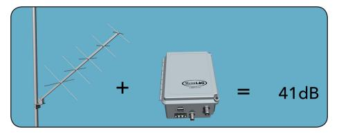
an 8dB Top Hat antenna, or a 4dB gain Omni antenna. The H-2221 V2 transmitter will adjust its output power based on the antenna type selected in order to maintain the proper level of effective radiated power. The options are listed below:
